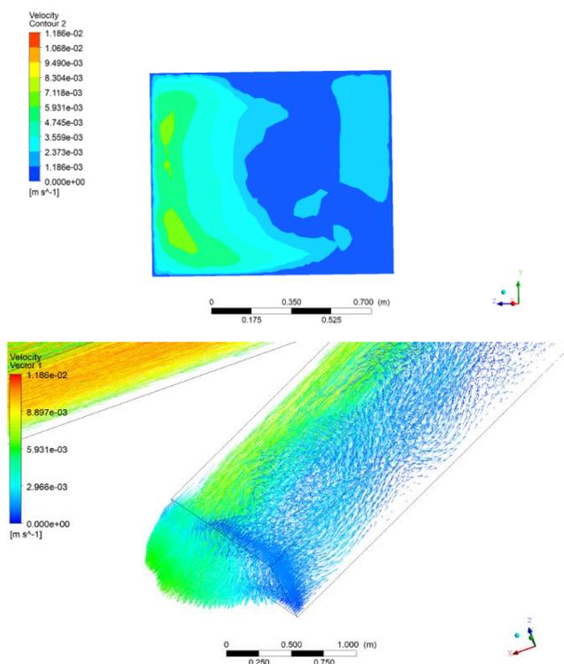
The above-mentioned figure represented that the majority of the flow line, contour, and the velocity vector has a concentration on the right face section of the intake canal. The design of the Vortex chamber was based upon the flow pattern result mentioned above. The below-depicted figure is of Vortex Chamber in which the turbine setup is to be installed.
