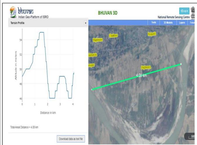
At location 4, the maximum available head is that of 9 meters, i.e. is the highest available head considered in this study for comparative analysis of low head turbines. The maximum power output here is 145.37 KW with a Kaplan turbine setup.
