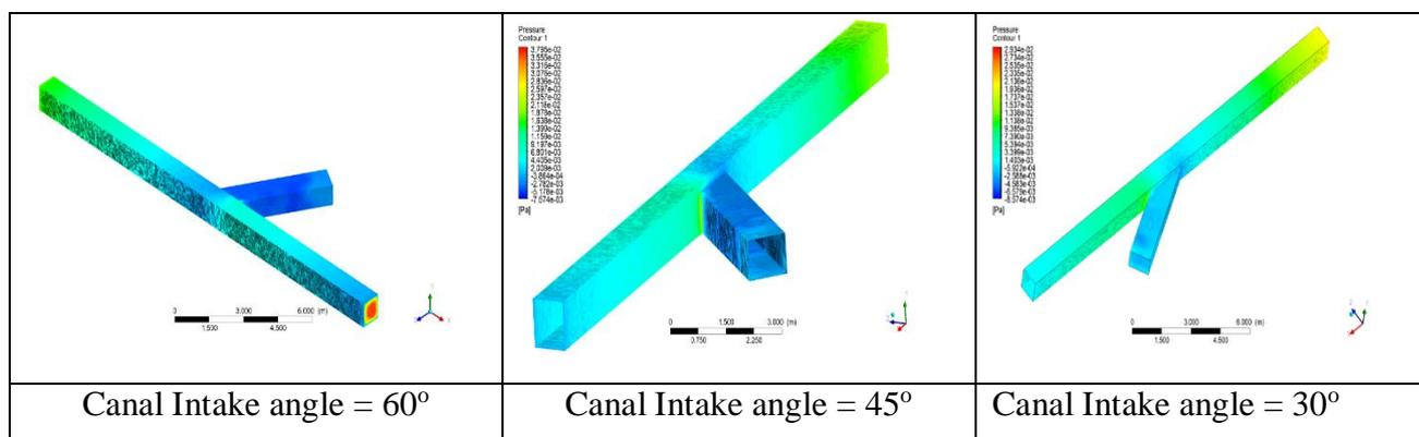
The canal intake angle having 30o inlet from the mainstream canal has maximum streamline flow traveling on the Right face of the Intake canal, resulting in the conceptual design of providing an inlet to the vortex chamber on the right side section. The graphical representation is mentioned below:
