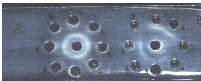
Figure 3. Interaction of total lectinic extract (A) with culture filtrate from T.reesei (1-4), B.subtilis (5) and the enzymes obtained after affinity chromatography on Raphanus lectins: from T.reesei (6-7) and B.subtilis (8). In B are presented the interactions of the same samples with one of the Raphanus lectins: that with fucose specificity.
