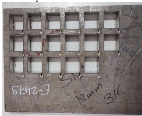
Fig. 1: Plate machined on fiber laser
